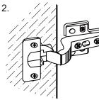
MOVE DOOR OUTWARD by turning this screw counter-clockwise KEEP DOOR IN RIGHT POSITION
